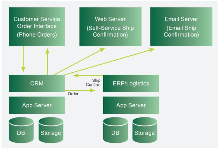
Figure 8 – Reference architecture for retailer that combines CRM and ERP for order processing.
