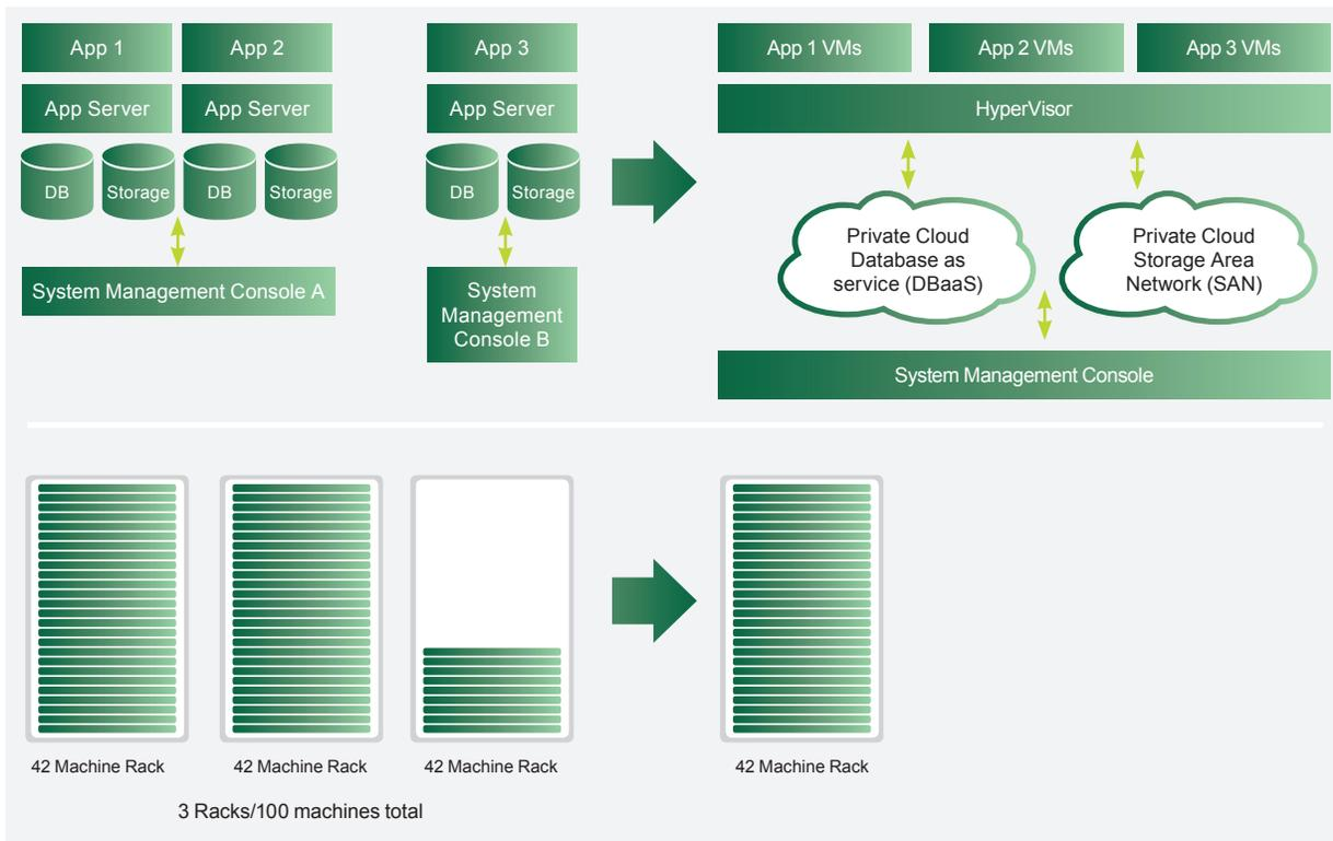
**Figure 12** – Example of server consolidation through virtualization. Separate database and storage systems for each application are merged into cloud-based database-as-a-service (DBaaS) and storage area network (SAN). One system management console can monitor the new virtualized environment. Chart for illustration only.
